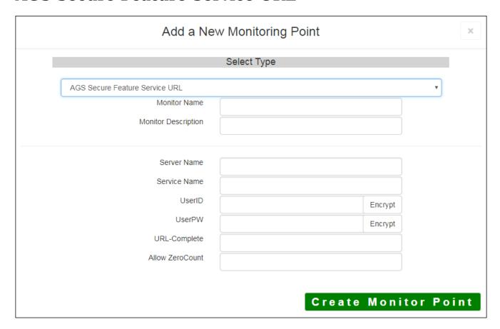
The AGS Secure Feature Service URL monitoring point checks an ArcGIS Server Secure Feature service for layer data and provides a count of the number of records returned.
