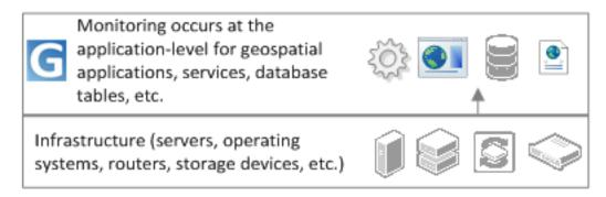
While this design does not specifically monitor an organization's infrastructure, it can assist with troubleshooting issues within the infrastructure by providing a focused list of applications that are affected.
