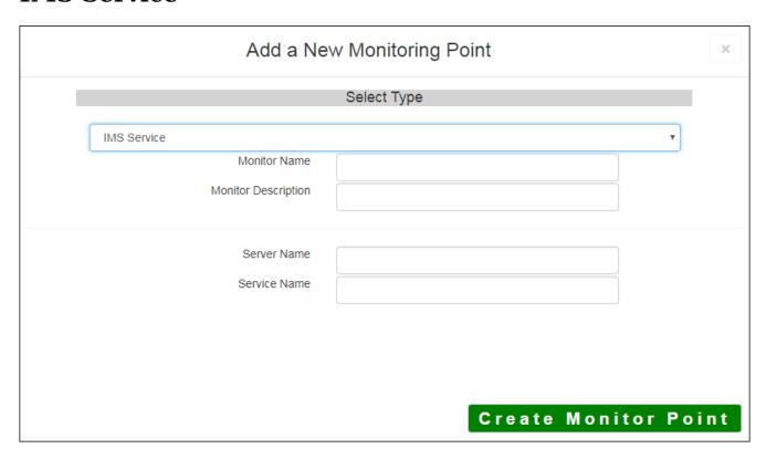
The IMS<sup>TM</sup> Service monitoring point performs three (3) checks at once. The first check makes sure the Esra active. The second check makes sure the ArcIMS<sup>TM</sup> catolog contains the service, and the third check confirmative.
