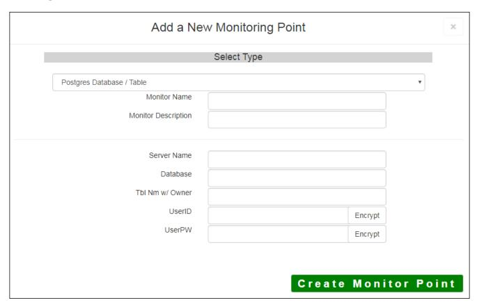
The Postgres Database/Table monitoring point makes an ODBC connection to the Postgres Database and checks if the Table is accessible and contains information.
